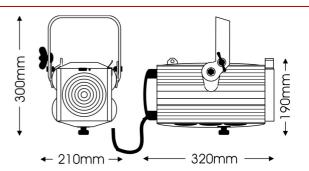
70W version of the popular architectural fresnel luminaire. Soffio f70 features a stylish body, a built-in ballast unit and compact dimensions. Ideal for display lighting and theatrical-style illumination of architectural spaces, the Soffio Fresnel produces a bright soft-edged beam, variable from 7° to 63°, shaped using an optional 4-leaf barndoor accessory.
