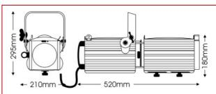
Ideal for closer-range highlighting, this 20°-40° profile spotlight uses a compact 70W discharge lamp combined with a double-condenser optical system to project a crisp flat beam particularly suited for projecting patterns or advertising logos in architectural and display applications. The cool beam design enables a wide range of metal, dichroic or acetate gobos and slides to be used.
