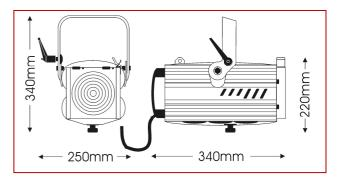
High power discharge Fresnel spotlight for display and internal architectural lighting applications. Suono f250 can use either a 250W MSD or a 300 MSA lamp and produces a softedged beam with a variable beam angle ranging from  $7^{\circ}$  to  $63^{\circ}$ .
