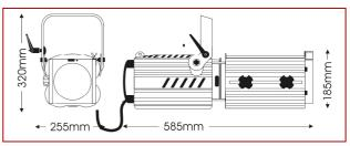
The wider-angle Suono D profile spotlight has a variable zoom focus from 20° to 40°, making it suitable for short-throw applications. The 250W MSD or MSA lamp produces a high-power 'daylight' beam which is popular for display, retail and architectural lighting.
