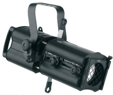
This versatile 500W/650W profile spotlight, designed for shorter throws, has a double condenser zoom focus optical system to provide crisp projection of gobos and a brilliant flat beam of between 20° and 40°. Features include a rotating gate, insulated rear handle, hinged lamp tray and double-microswitch interlock for safe lamp replacement.
