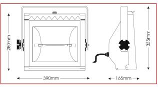
Also for larger venues, this 1000W symmetric floodlight produces a wide, even wash of light for general lighting purposes. Each unit is complete with a safety glass and a double microswitch interlock for safe lamp replacement. The modular design enables several units to be coupled together to form a compartment batten.
