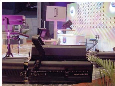
A high-specification 1000/1200W profile spotlight with advanced features including a double condenser optical system for extremely sharp gobo projection, rotating 4-shutter gate, 8° to 22° narrow-angle zoom focus, a double-microswitch interlock for safe lamp replacement, easy access for lens cleaning and a cranked fork. Ideal for front-of-house projection positions.
