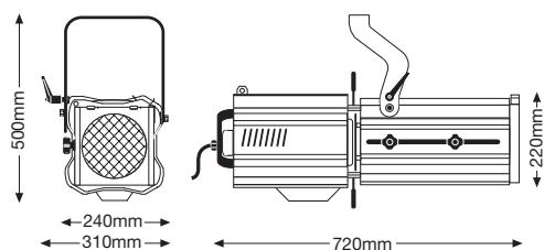
For closer projection in larger venues, this wide-angle 18° - 36° 2000W spotlight incorporates a zoom focus double condenser optical system, rotating gate, a cranked fork and a double microswitch interlock for safe lamp replacement.
