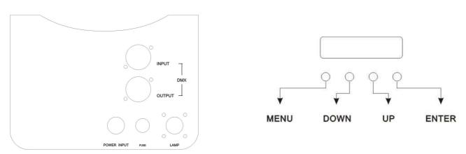
(1) Setup of initial address: press ENTER button, the heading A will not be shown in the address code display, indicating it's already in the address setup state; press UP/DOWN to increase or decrease the address code till the required code, and press ENTER to save it (no need set address code after each power on).
