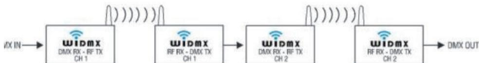
Receiver and transmitter connected directly, and working with different grouping or connection, can act as a repeater or amplifier, can increase the effective working distance.
