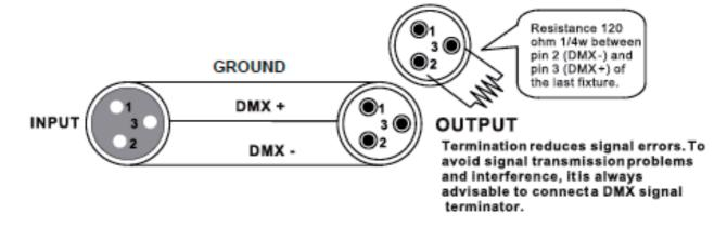
**Caution:** Do not allow contact between the ground and the fixture's chassis ground. Grounding the ground can cause a ground loop, and your fixture may perform erratically. Test cables with an ohm meter to verify positive pole and to make sure the pins are not grounded or shorted to the shield or each other.
