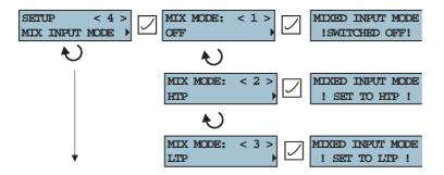
The dimmer is switched to the HTP or LTP mix mode now. In this mode, the dimmer is controlled via DMX and 0-10V input at same time.
