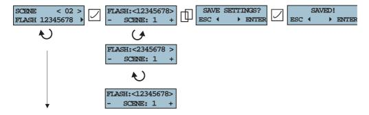
The flash scene is a scene mode, where scenes are called by a single press of button. When any other button on HLC is pressed, the other scene is called. You can preset up to 8 scenes. A scene that is to be Flash must be added to the Flash scene list. Turn the Encoder until you get to the desired scene number and confirm by ENTER button. To remove a scene from the Flash scene list, turn the Encoder to the scene number and press the ESC button. A single press of the Encoder saves all settings.
