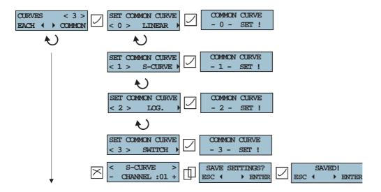
Press the left button to select the curves for each channel individually or the right button to set one common set of curves for all channels.
