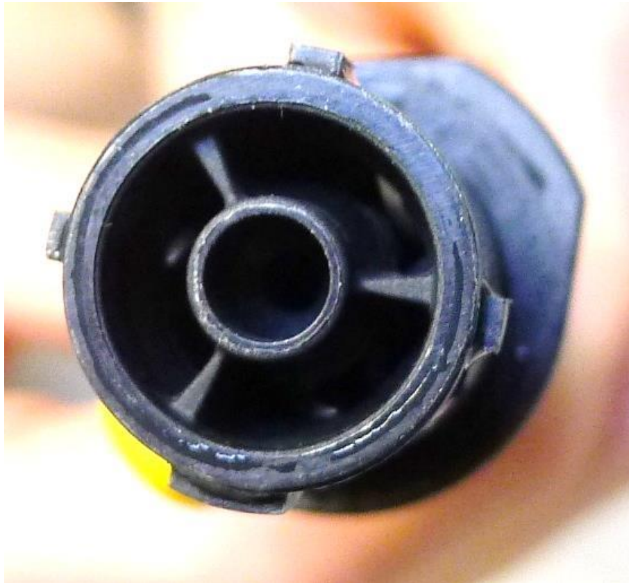
After IP65 test: No water and no dust entered
