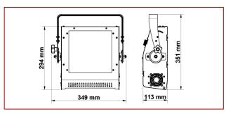
120 watt LED RGBW asymmetrical floodlight ideal for cyclorama-type lighting in all applications.
