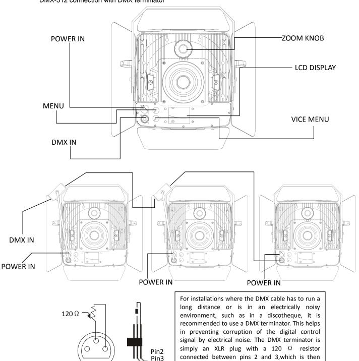
plugged into the output XLR socket of the last fixture in the chain. Please see illustrations below.
