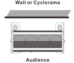
Note: The direction of light can be changed by changing the direction of the lenses.
