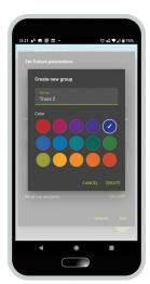
You can also choose to add the fixtures to a group. A group enables you to control the common parameters of several fixtures simultaneously or step through the fixtures in sequence.
