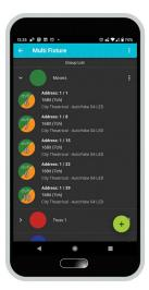
In the Group List, you can click on a group to control the common parameters of all of the fixtures in that group (for example a group containing different models of moving lights will likely have at least intensity, pan, and tilt in common).
