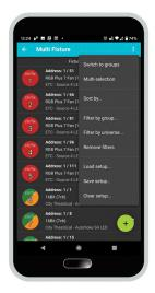
When you have completed patching, you will be presented with the list of fixtures in your setup. Their fixture number will contain the colors of any groups they belong to. You can either select fixtures to control or press the 3-dot menu for more options including sorting, filters, saving the current setup or load a pre-existing one, and switching to the group view.
