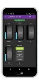
When you select an individual fixture from within the group you will be controlling just that fixture, but you can step through the fixtures in the group using the right and left arrows. The attributes you change will transfer to the new fixture enabling you to quickly step through the group to test your fixtures.
