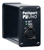
The Portable Uno may be powered using Power-over-Ethernet or a 24VDC supply with a 2.5mm center-positive barrel connector.
