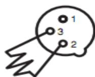
Termination reduces signal errors and avoids signal transmission problems and interference. It is always advisable to connect a DMX terminal, (Resistance  $120\Omega$  1/4 W) between PIN 2 (DMX-) and PIN 3 (DMX +) of the last fixture.
