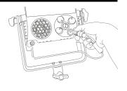
Insert the DC XLR 4 pin connector into the input jack on the SUPERPANEL 30 and power on the fixture.
