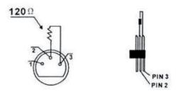
**Caution:** At the last fixture, the DMX-cable has to be terminated with a terminator. Solder a 120 resistor between Signal (–) and Signal (+) into a 3-pin XLR-plug and plug it in the DMX-output of the last fixture.
