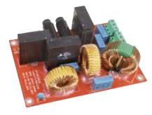
[ \* all fixtures of this series ] High immunity to voltage overloads thanks to the use of a 10KV-20KA Surge Protection Module capable of withstanding voltage and current pulses up to 10.000Volt and 20.000Ampere.
