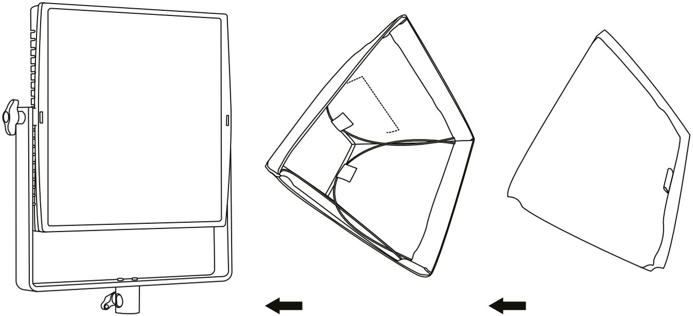
To secure the softbox at the Superpanel 30 pass the velcro string at the edges of the panel and make sure to tighten it. (fig 1)
