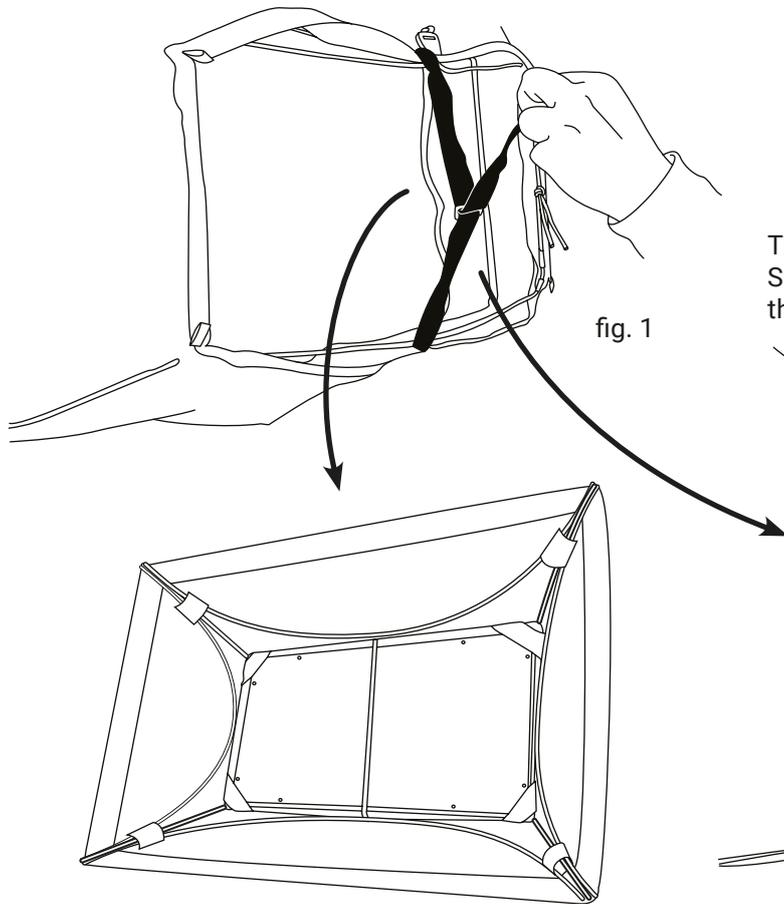
The black velcro string goes to the back of the Superpanel and the white elastic string goes to the front to fix tightly the softbox. (fig 1)
