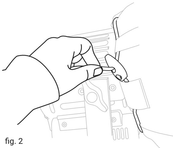
Tighten the elastic to close the gap between the softbox and the Dayled PRO until it's fixed (fig. 2).
