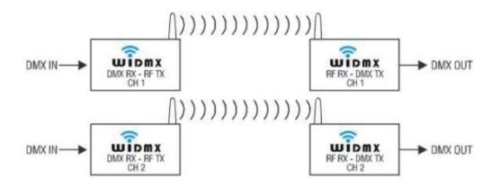
Plural sets of radio transmitters can be operated simultaneously, without disturbing each other.
