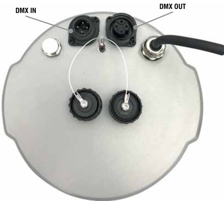
Female and Male 4 PIN connector / Connettore 4 PIN femmina e maschio
